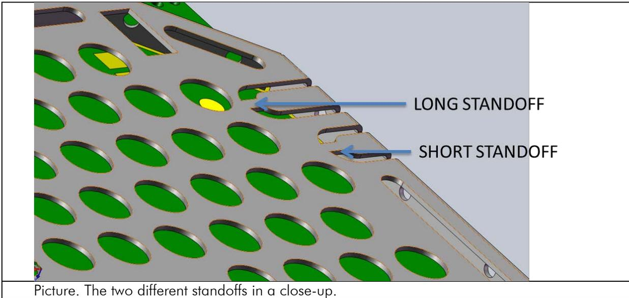
Picture. The two different standoffs in a close-up.
