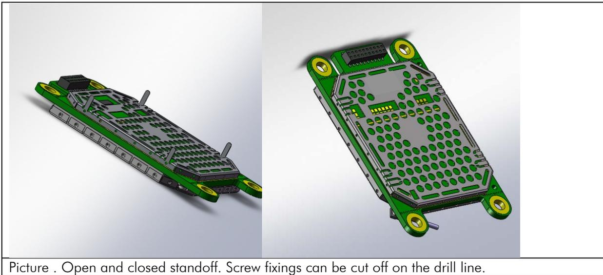
Picture . Open and closed standoff. Screw fixings can be cut off on the drill line.
